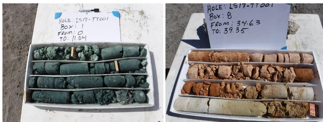
Figure 10-3: Drill core presented prior to sampling procedures, showing examples of green clay, orange clay, and limestone typical of La Salada salar material
