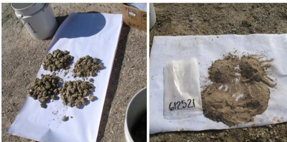
Figure 6-1: Coning and quartering method to collect representative samples for analysis by Litio Mex at Caligüey
