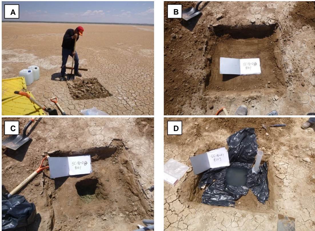
Figure 9-12: Photographs showing pit and water method for density sampling
