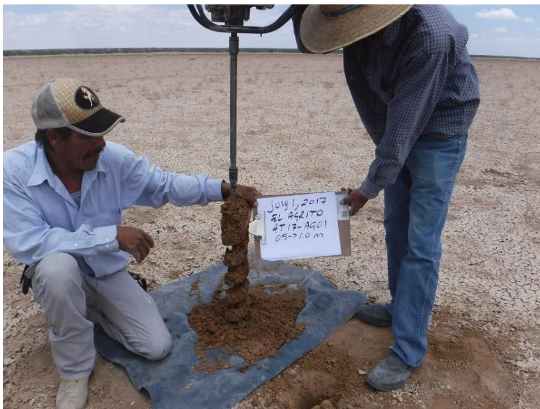
Figure 9-1: Example of surface sediment sampling by hand-auger 2017
